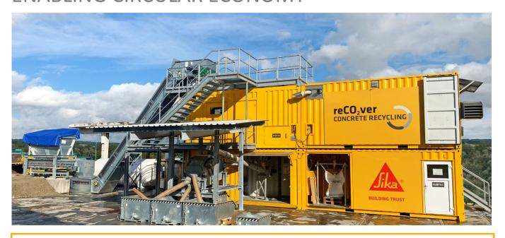
Segregates concrete back to its original ingredients to be re-used for new high-grade concrete
