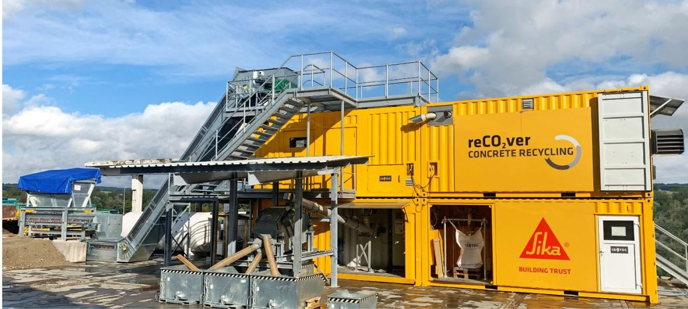
**Segregates concrete back to its original ingredients to be re-used for new high-grade concrete**
